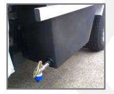
Underslung Water Tanks Food Grade Tanks with locking tap available in center or side mount Configurations - Side Mount -45LCenter Mount - 50L
