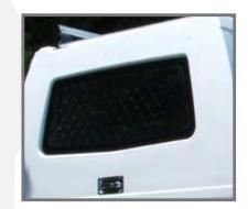
Front and Rear Windows 4mm Toughened Safety Glass providing the most visibility available on a service body.
