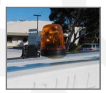
**Rotating Amber Beacon** 12 volt rotating amber beacon with dashboard switch
