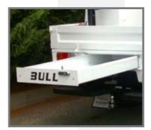
Slide Out Drawer Available in unsealed or sealed versions at lengths of either1.5m or 1.8m. Provides storage space for shovels brooms etc.
